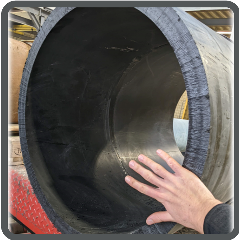
A thick 800mm pipe that the PE Pipe Cutter cut in just over 5 minutes
