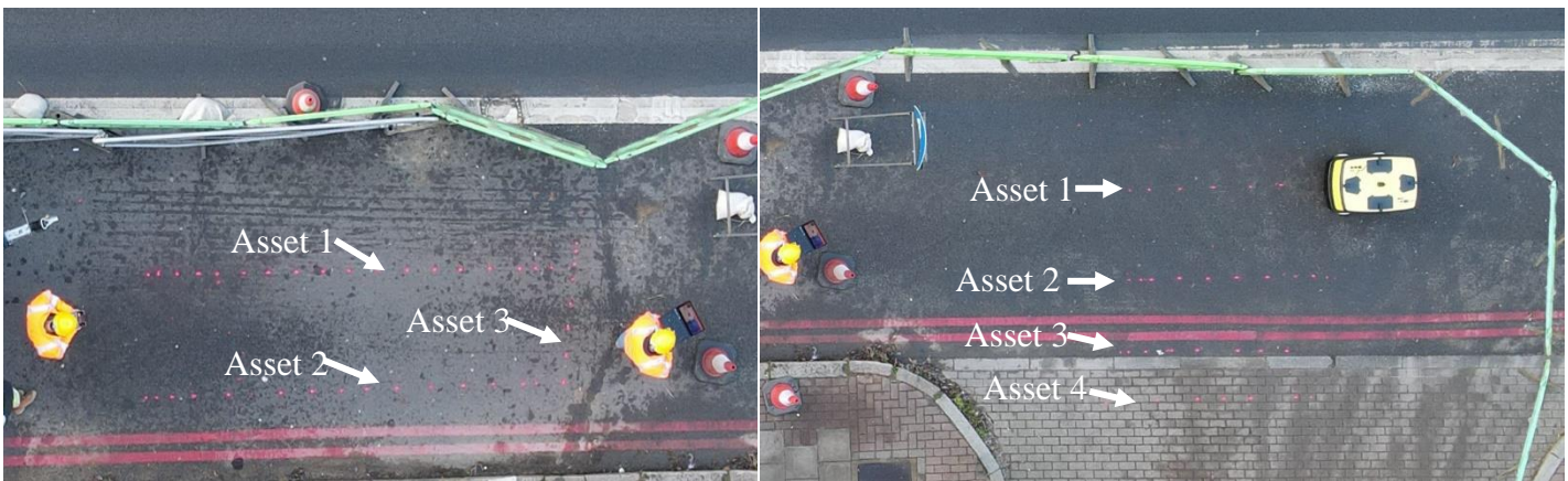
Figure 5: Same-day mark-out performed by AUSMOS at Clapham
