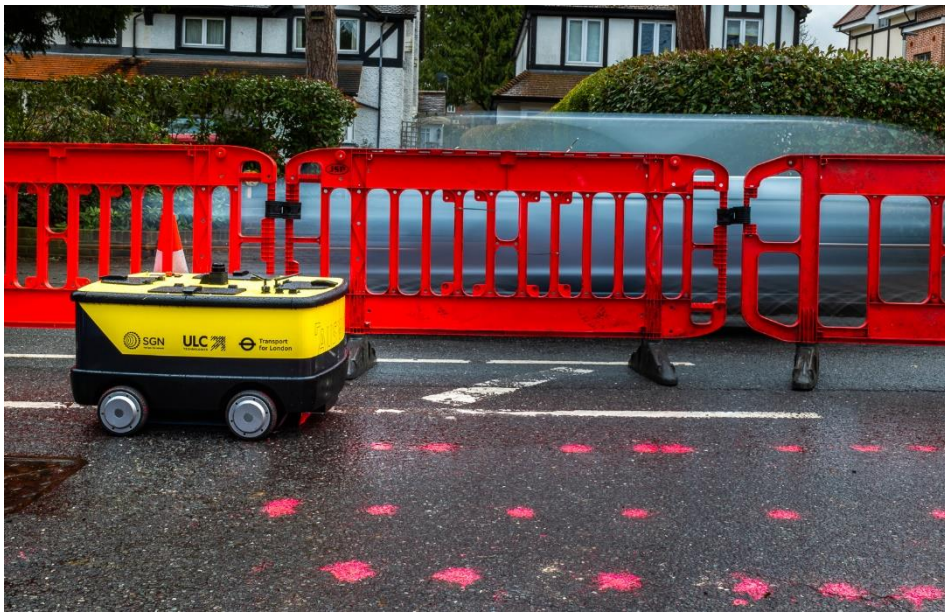
Figure 1: AUSMOS scan and mark-out
