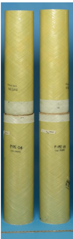
Figure 4 Two Fully Thermoplastic Welded/ Assembled Glass Reinforced Thermoset Pipes (8" Pipe, 2m Demonstrator)
