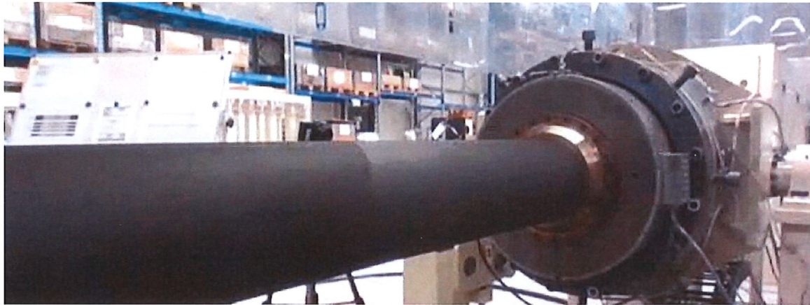
3. Extrusion of the weight coating at Strohm's 24/7 plant in The Netherlands
