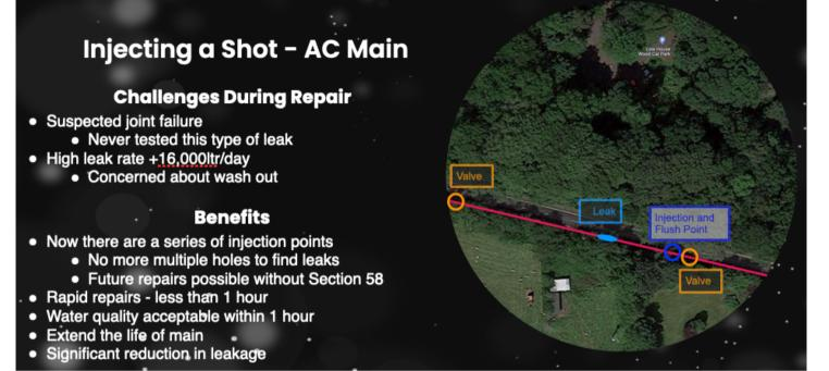
The challenge with this repair is the leaks are frequent, are always nonvisible, and often significant. The road has just been resurfaced and so resurfacing costs are high and traffic management essential. It is now possible to repair future leaks without traffic management and it will be possible to extend the life of this asset.
