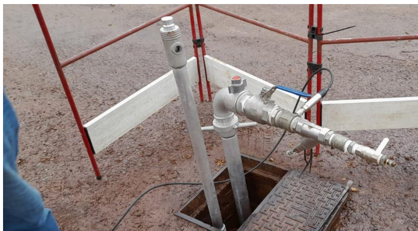
Wave generation point with monitoring transducer.
